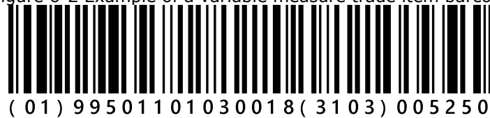
Figure 6-2 Example of a variable measure trade item barcode
