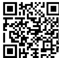
Figure 5-22 Example of GS1 QR Code symbol encoding a GTIN AI (01) and extended packaging URL: AI (8200)
